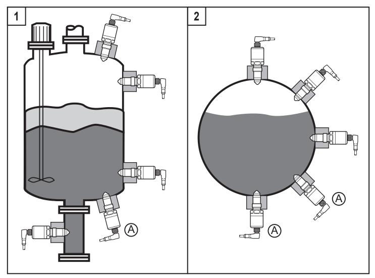
The unit can be installed at any position.
